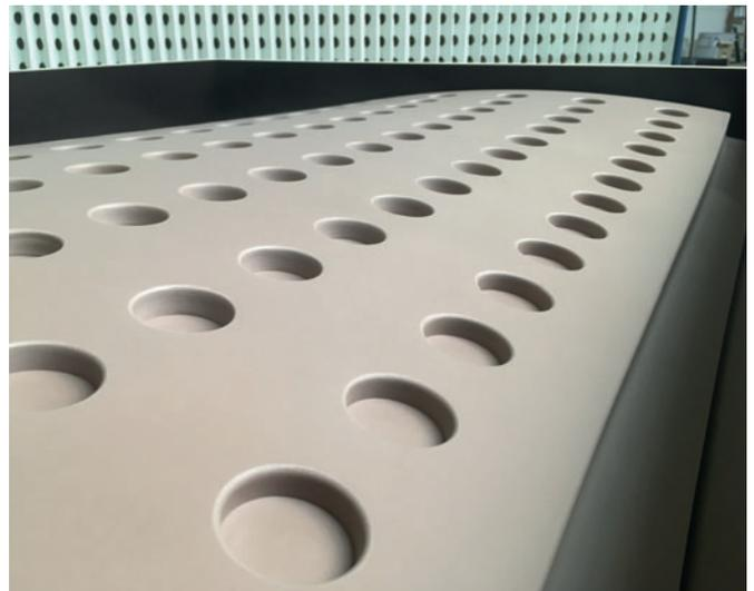
*The surfaces of the models are smoothed following the CNC machining. The models are given a micro-fine coating for a smooth and closed surface.*
