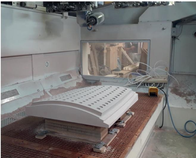
*Wasa uses a CNC 5-axis portal milling machine to manufacture the models.*
